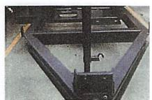
I BEAM TRAILER. Units are built from start to finish at our factory, including the trailer which consists of a sturdy I beam construction.
